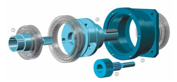
Total reduction ratio between the sun gear and the output shaft is: 1+Z3/Z1. It is an exact number, which means the number of rotation of the output shaft is exactly proportional to the number of rotation on the input shaft. However, within one rotation, the angular position of the shaft cannot be considered exact, its precision depends on the precision of the inner elements of the gearbox and is more or less equivalent to the backlash.
